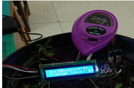
Gambar 6. Pengujian *Soil Moisture* Dengan Alat Ukur *Soil Moisture*
