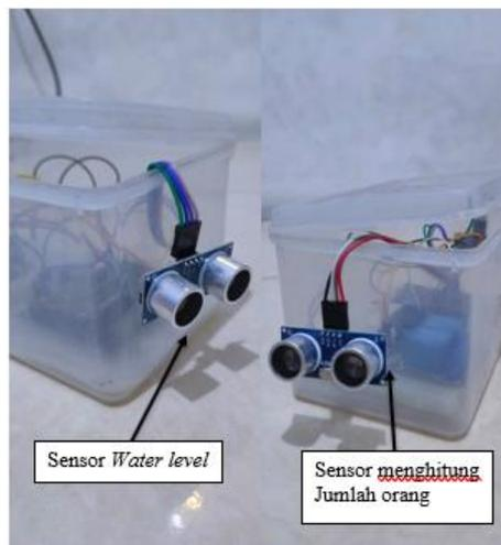
**Gambar 6** Rangkaian Sensor Ultrasonic
