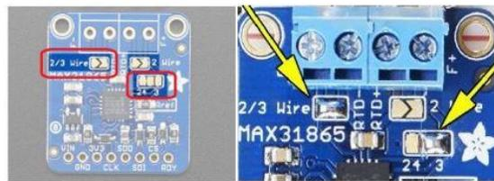
**Gambar 10** Setting PT100 3 kabel
