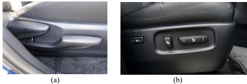
Figure 1. (a) Manual Mechanism; (b) Automatic Mechanism
