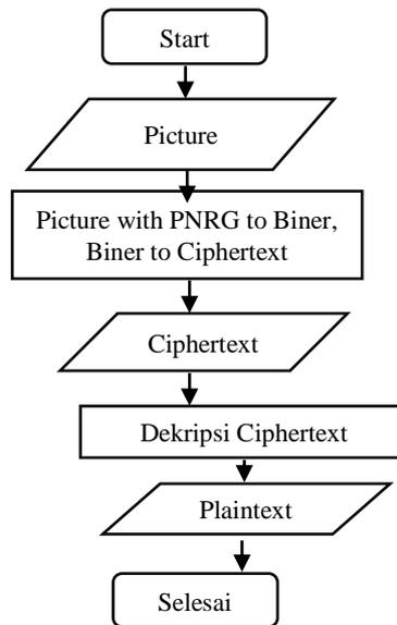
**Gambar 4 Flowchart Proses Dekripsi**
