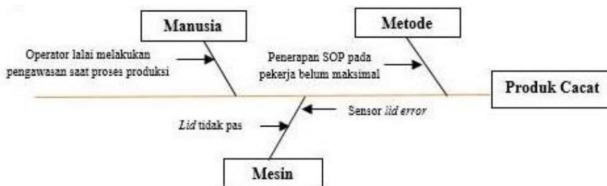
Gambar 3. Fishbone Diagram Cacat Jenis Lid Miring
