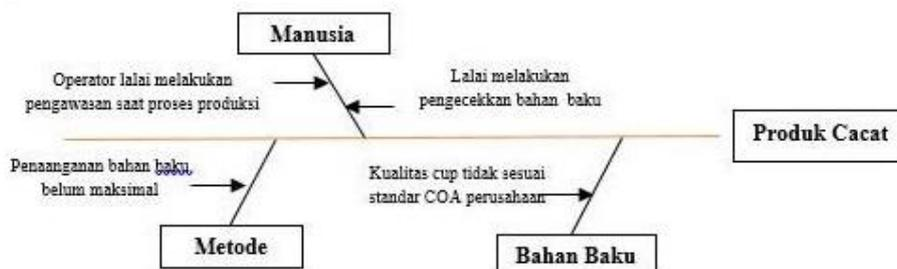
Gambar 5. Fishbone Diagram Cacat Jenis Cup Bocor
