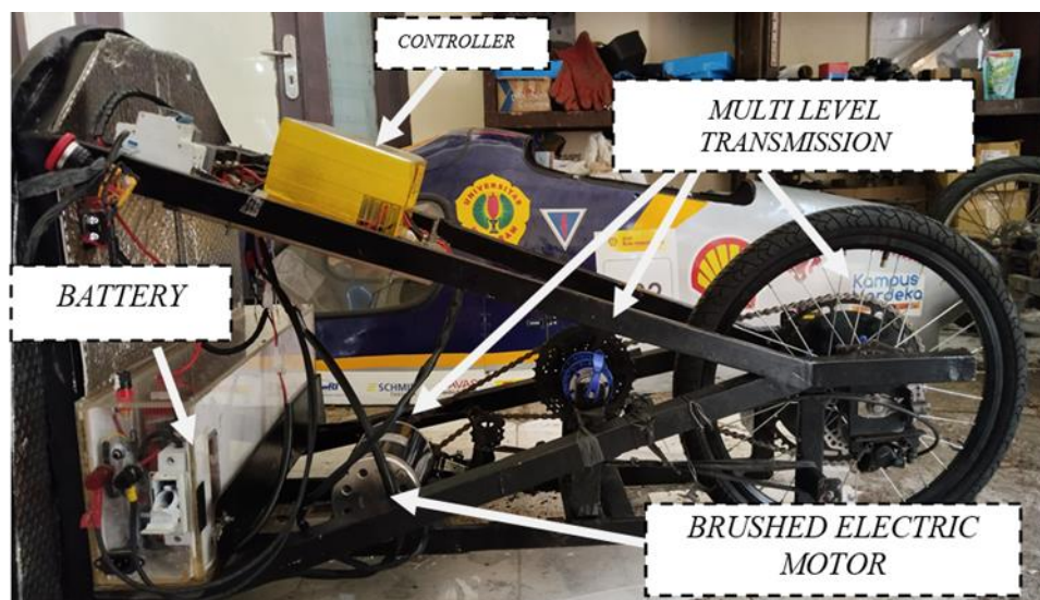
Figure 1. A prototype electric vehicle was used for field testing to evaluate the effects of vehicle weight and gear ratio on energy consumption, as previously demonstrated in a related study [22].
