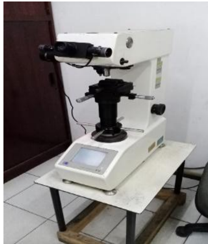
Figure 2. A Mitech HVS-50AT micro-Vickers hardness tester was used for the hardness measurements.
